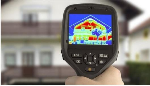
Thermal imaging in every room and the attic to identify sources of thermal losses due to problems with insulation and air infiltration as well as leaks in the HVAC ducting, overloaded electrical wiring, and even water leaks on flooring, walls, and ceilings.
